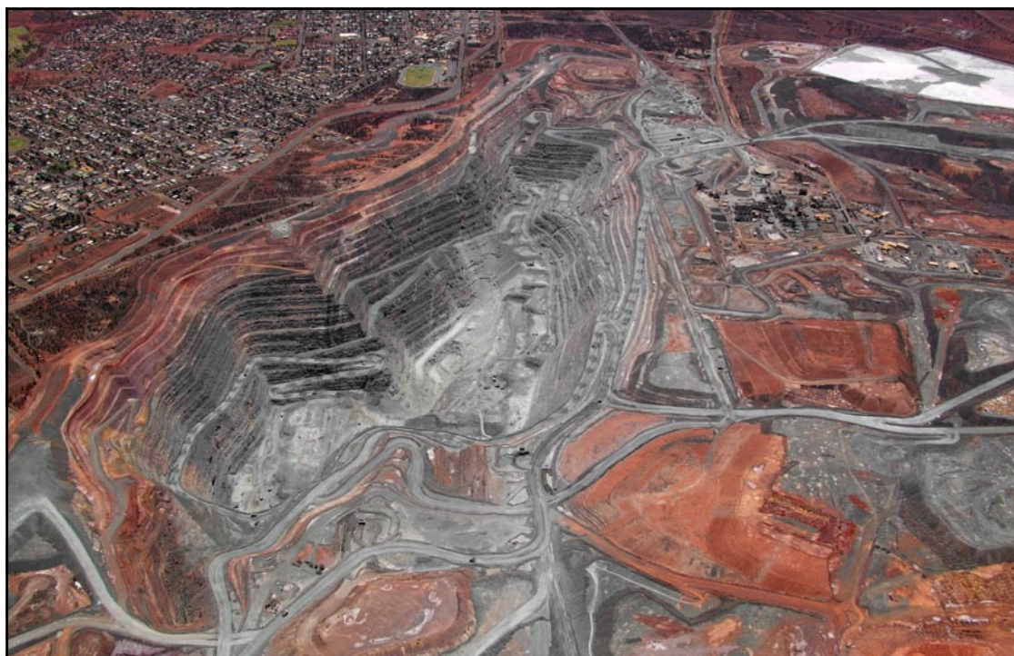
Figure 26. The Superpit that is now extracting gold from the entire zone of veins at Kalgoorlie; the town is at top left, and the mineral processing plant and waste tips are on the right (photo: KGMA).
